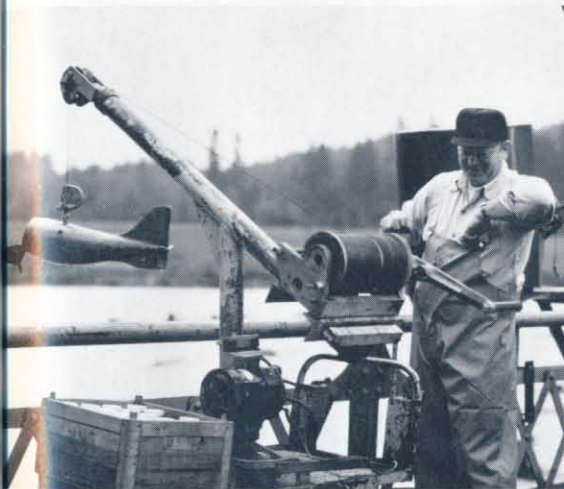
U.S. Geological Survey scientist Al Onions taking suspended sediment samples along Highway 99 near Castle Rock, Washington, on December 5, 1982.
