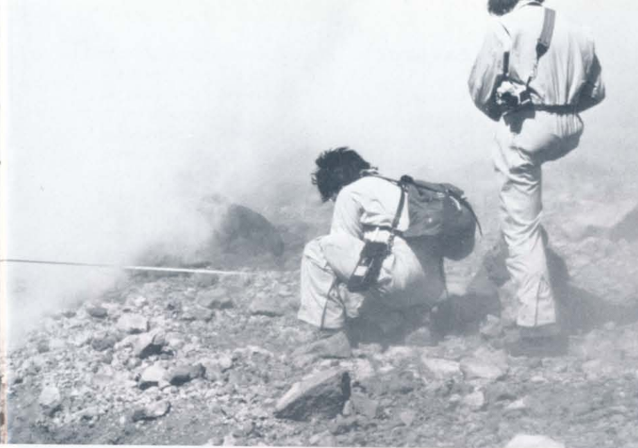
moved several meters. Measurements of radial cracks and thrust faults were extremely important in predicting the 1981 and 1982 dome-building eruptions, but, during the 1983 "continuous eruption," the dome became too large, and talus from the dome covered the crack and thrust areas.
