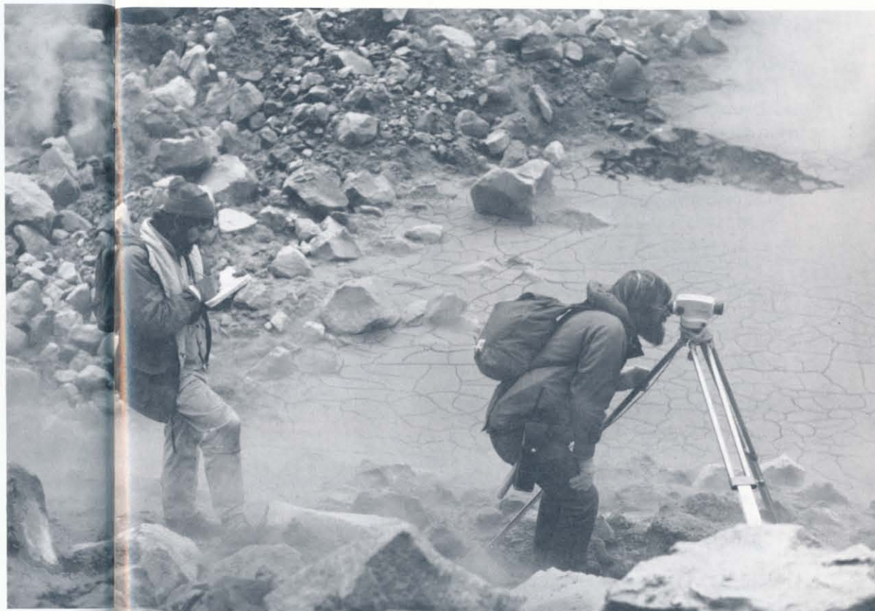
U.S. Geological Survey personnel leveling around Mount St. Helens dome on November 6, 1981. Repeated leveling circuits around the dome have been performed to determine possible changes of the crater floor before eruptions.
