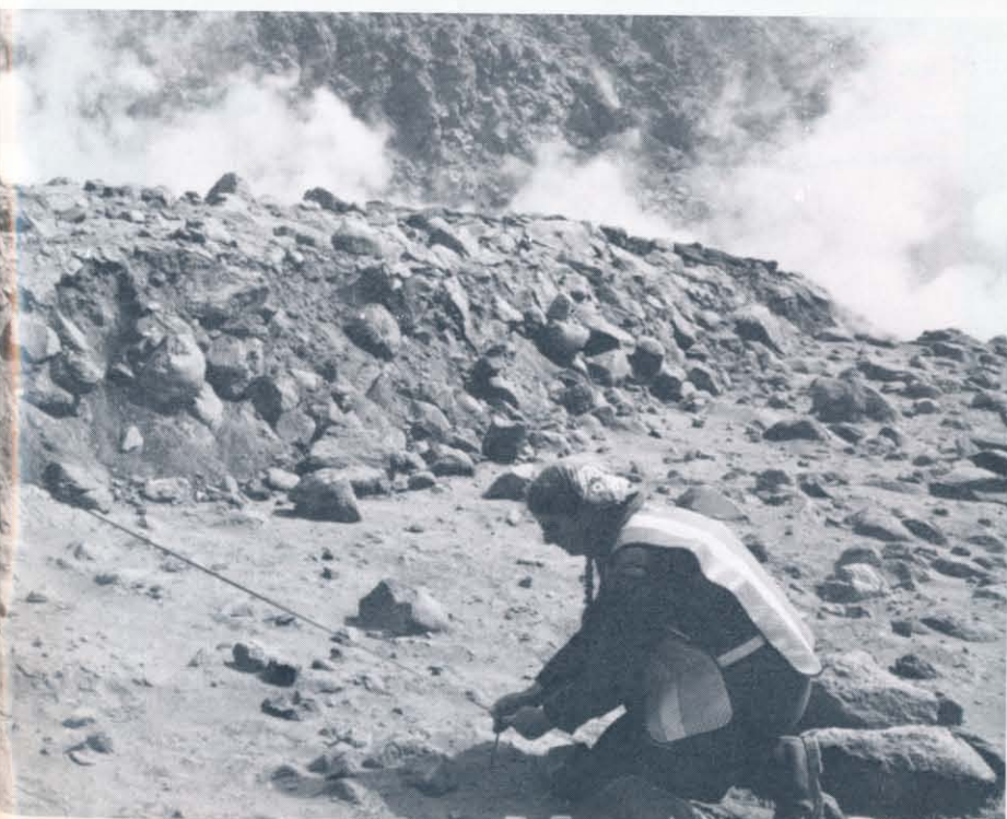
moved several meters. Measurements of radial cracks and thrust faults were extremely important in predicting the 1981 and 1982 dome-building eruptions, but, during the 1983 "continuous eruption," the dome became too large, and talus from the dome covered the crack and thrust areas.
