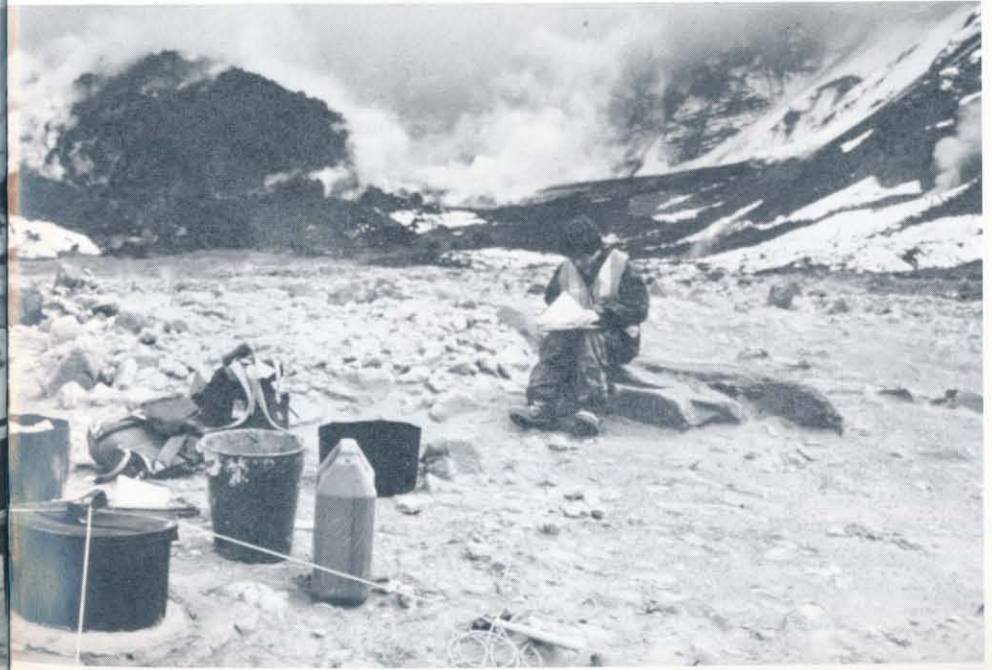
Electronic tiltmeter site, north of dome, April 1981. Tilt measurements record changes in the inclination of the ground surface on the crater floor and around the dome. A network of electronic tiltmeters and spirit-level stations in the crater has been used to help monitor deformation before and during eruptions. These records of changes in the inclination of the ground have been useful for predictions; electronic tiltmeters installed on the crater floor detect changes several weeks before an eruption, and the rate of change begins to accelerate rapidly several hours to several days before an eruption. (Photograph by Terry Leighley, Sandia Labs.)
