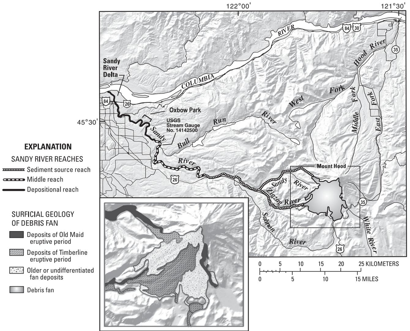
Figure 1. Location map for the Sandy River at Mount Hood, Oregon. Sediment-source, middle, and depositional reaches of the Sandy River are indicated. Inset map is a simplified geologic map of the debris fan (modified from Scott et al., 1997a), showing recognized deposits of Old Maid and Timberline age (the two late Holocene eruptive periods) on and just downstream of the fan surface. Old Maid sediments also entered the White River drainage (not studied), but none entered the Hood River drainage.
