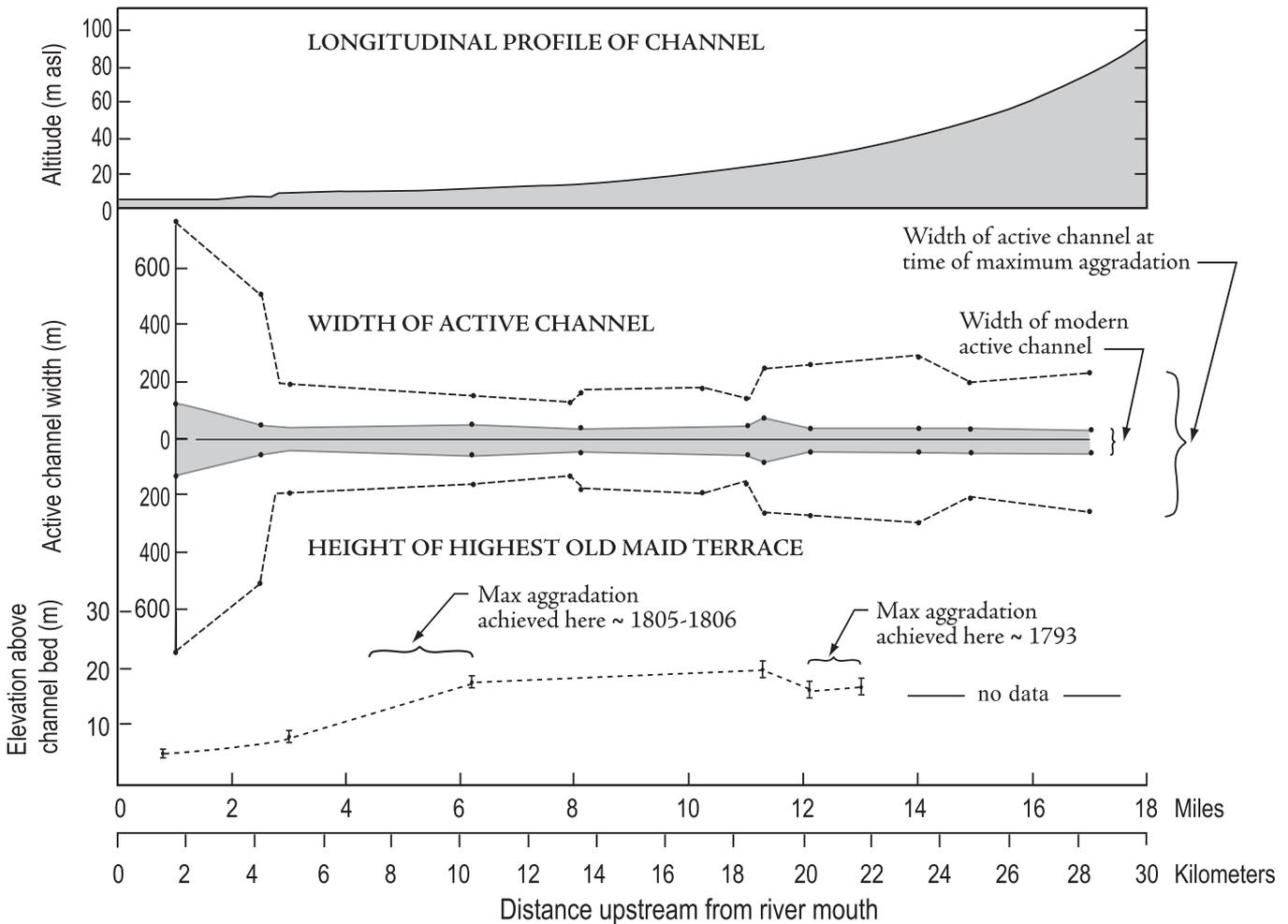
**Figure 10.** Valley morphology and terrace height in the lowermost 30 km of the Sandy River, downstream from Mount Hood. In this plot, the depositional reach extends from 0 to 26 km. The first 4.7 km of channel are on the unconfined Sandy River delta. Width of active modern channel is approximate, based on width measured from a 1952 U.S. Geological Survey topographic map.
