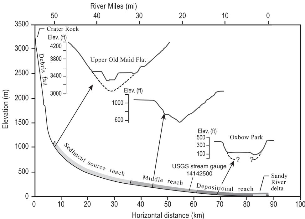
**Figure 4. Longitudinal profile of the Sandy River channel, starting at Crater Rock (source volcanic vent) and continuing down to the Sandy River confluence with the Columbia River. River reaches described in the text are indicated, and selected valley cross sections for each reach are shown. Profile data were derived from U.S. Geological Survey (USGS) 30 m digital National Elevation data set and USGS 1:24,000 digital line graph (DLG). Vertical exaggeration is 9.3x.**
