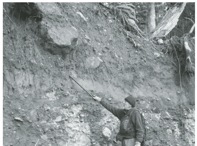
Figure 12. The distal end of the large Rainbow Creek debris avalanche is seen at Stop 5. Note the sequence of subrounded alluvium at the bottom, the prominent undisturbed soil layer (where Kevin Scott is pointing), and the poorly sorted debris avalanche deposit at the top.
