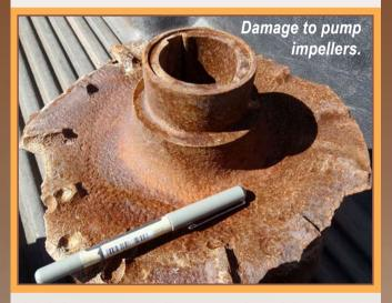
Ash-laden wastewater will cause accelerated damage to pump impellers including metal pitting and thinning. Photo by Carol Stewart.
