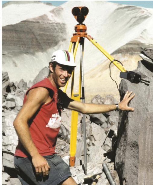
Jack Kleinman sets up an EDM reflector atop Novarupta dome in the Valley of Ten Thousand Smokes.
